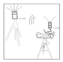
It is recommended that transmitter antennas shall be changed to cross-facing to the receiver, shown as below:
