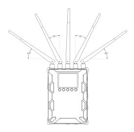
2.Connect the Receiver to the power supply via the certain power cable or V-mount battery. Connect the SDI/HDMI cable to the TV/Monitor.
