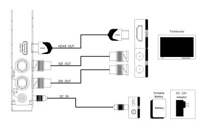
3. Turn ON the power supply and make sure the receiver start to work.
