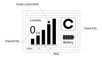
Screen Lock/Unlock : The screen will be always locked unless long press the MENU button to unlock.
