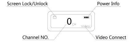
Screen Lock/Unlock: The screen will be always locked unless long press
