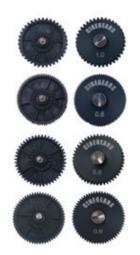
Cinegears 38mm Variety Pitch Replacement Gears are included, with the radius side of 38mm (original is 45mm), which can provide you with even smoother movement for small lenses. It also can work with different lenses with variety pitches. The pitch size includes: 1.0, 0.8, 0.6 and 0.5.
