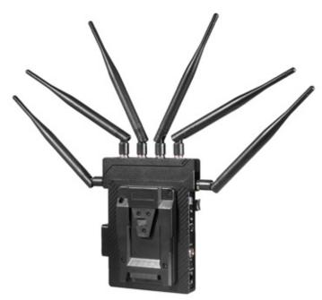
4. Setting the receiver higher will enhance the transmission distance.
